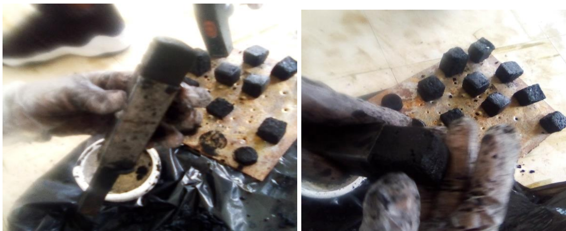
Figure3. 3: Molding of briquettes
