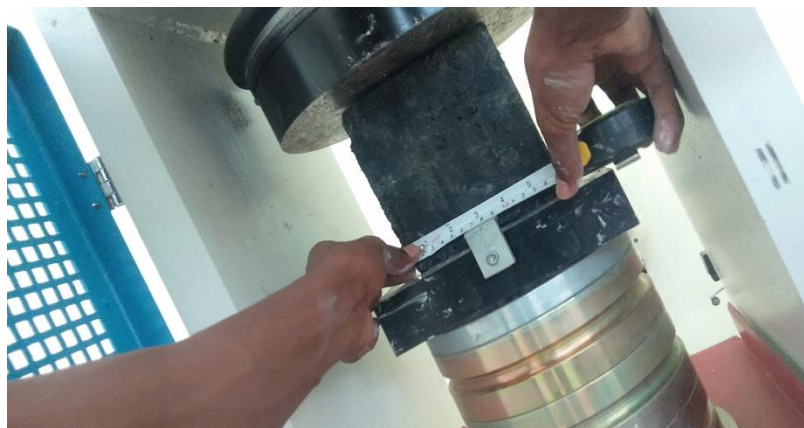
a) Checking perpendicularity of cube casted concrete
