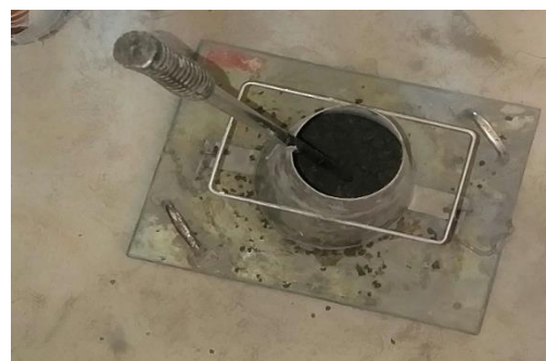
b) Preparing slump for test
