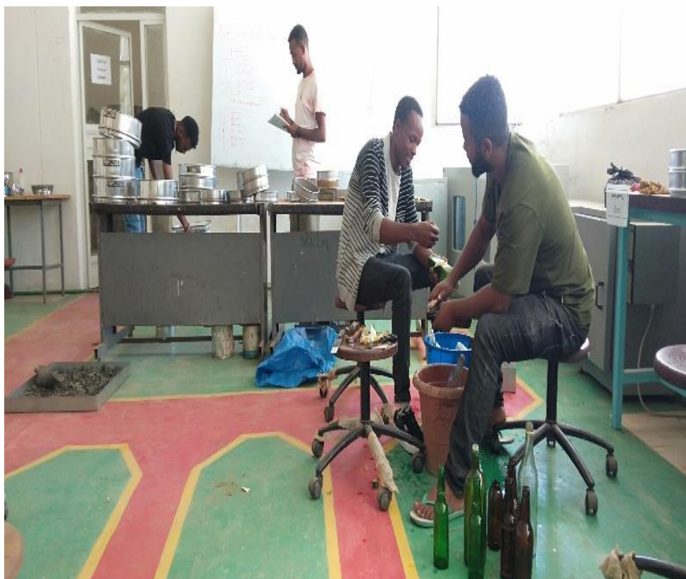
Figure 4 cleaning waste glass manually
