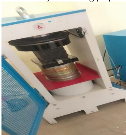
b) Preparing the concrete for testing
