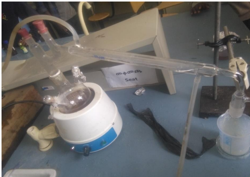
Figure 6 separation of fat from solvent by distillation
