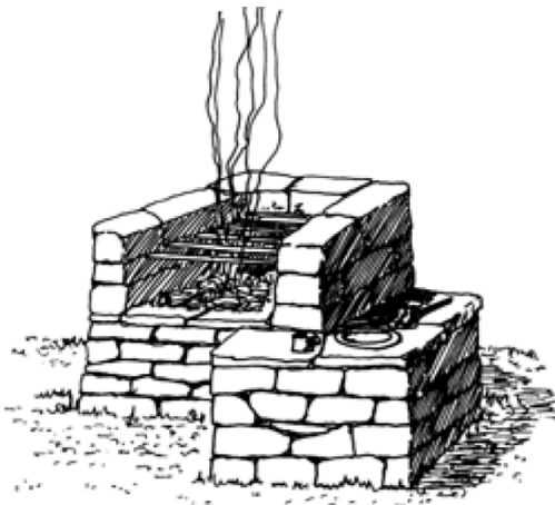
This design incorporates a fixed grill and a lower table on which to place plates, utensils etc.
