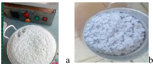
Figure 3.5 pulp after bleaching with chemical ( a) and (b) without chemical
