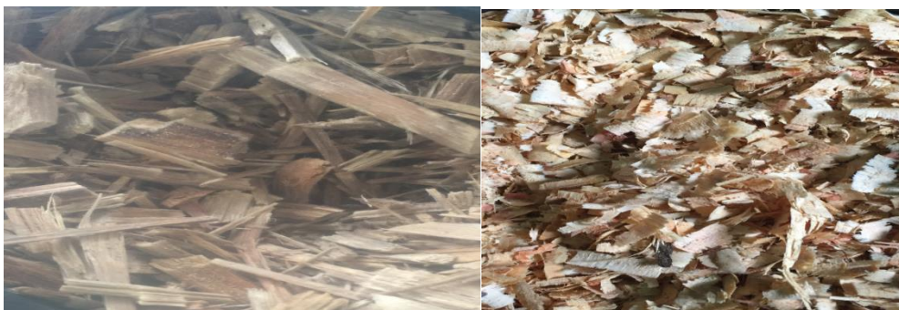
Figure 3.2 Size reduced by using Axes(A) and knife(B)
