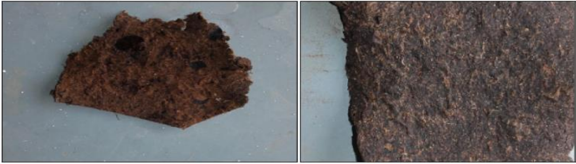
Figure 4.1 Bioplastic made from large size fiber
