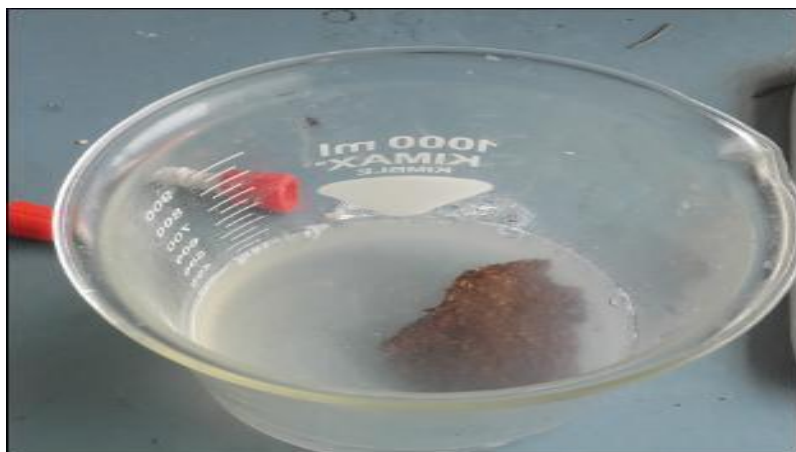
Figure 4.5. Solubility test of bio-plastic
