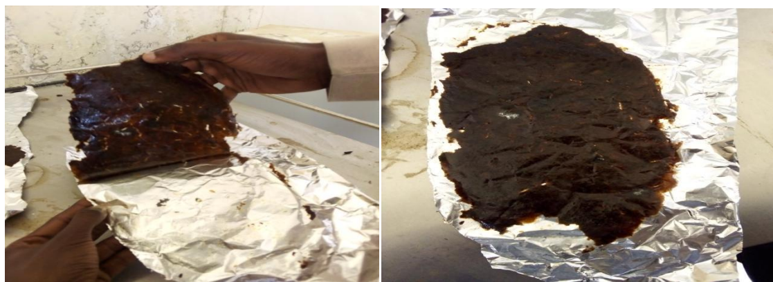
Figure 3.3 Film forming from banana peels
