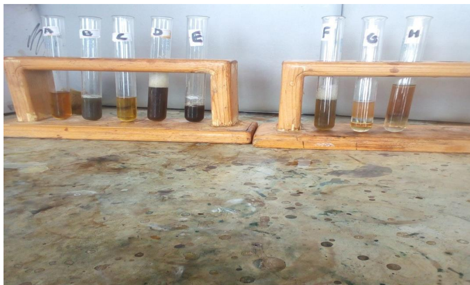
Figure 1: Phytochemical test result of Croton macrostachyus extract for (a) coumarins (b) tannins(c) glycoside, (d) flavonoid, (e) phenolic, (f) saponins, (g) steroid and (h) terpenoids, plant constituent metabolites [91].
