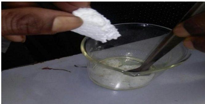
Figure 3.5 mixing of polystyrene with naphthalene.
