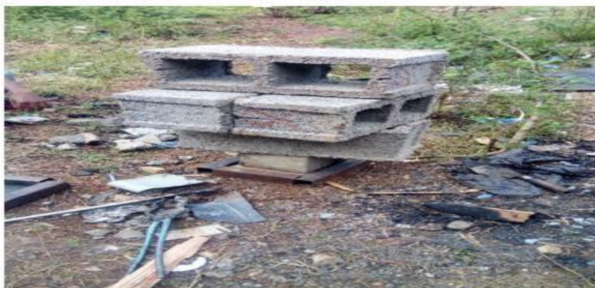
Figure 7 using weight as pressing load in production process
