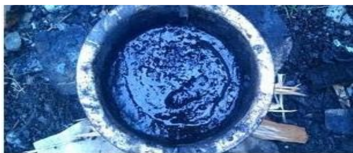
a) Melting (PET) plastic waste
