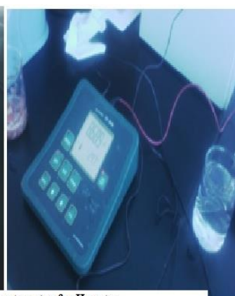
Annex Plate 10: Digital Refractometer & pH meter (used for TSS & pH measurement)
