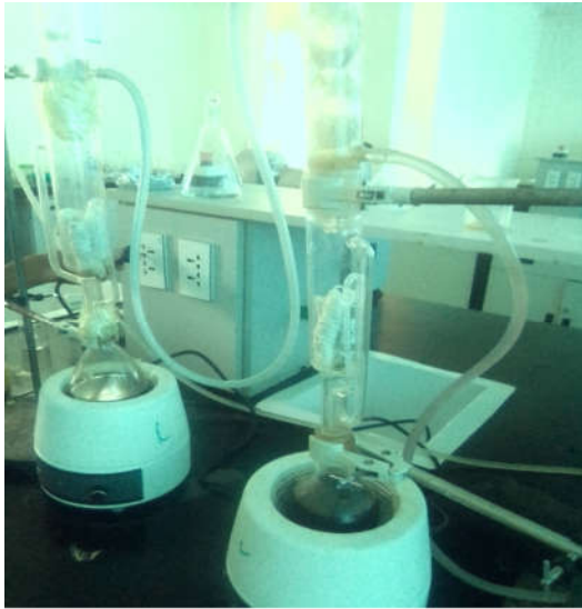
Appendix figure 13. Soxhlet apparatus when extraction of crude fat
