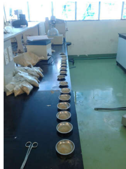
Appendix figure 12. Oven dried samples were ground and prepared before analysis begun
