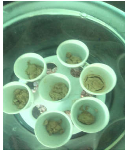
Appendix figure 14. Acid Detergent Fiber after dried out in oven cooled in Desiccator
