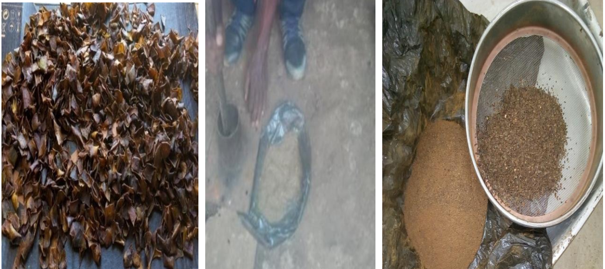
a) Dried Mango Peel b) grinding by using mortar and pestle c) sieving Figure 3.3. Dried Mango Peel. grinding by using mortar and pestle and sieving
