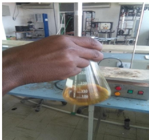
Figure 3.5 titration of oil to determine acid value
