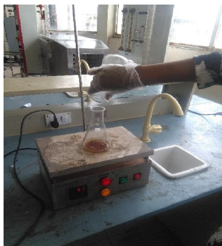
Figure 3.5 titration of oil to determine acid value
