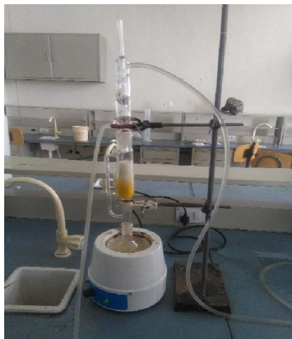
Figure 3.4 oil extraction using soxhlet extractor
