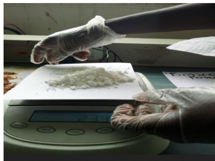
Figure 10. boric acid measuring
