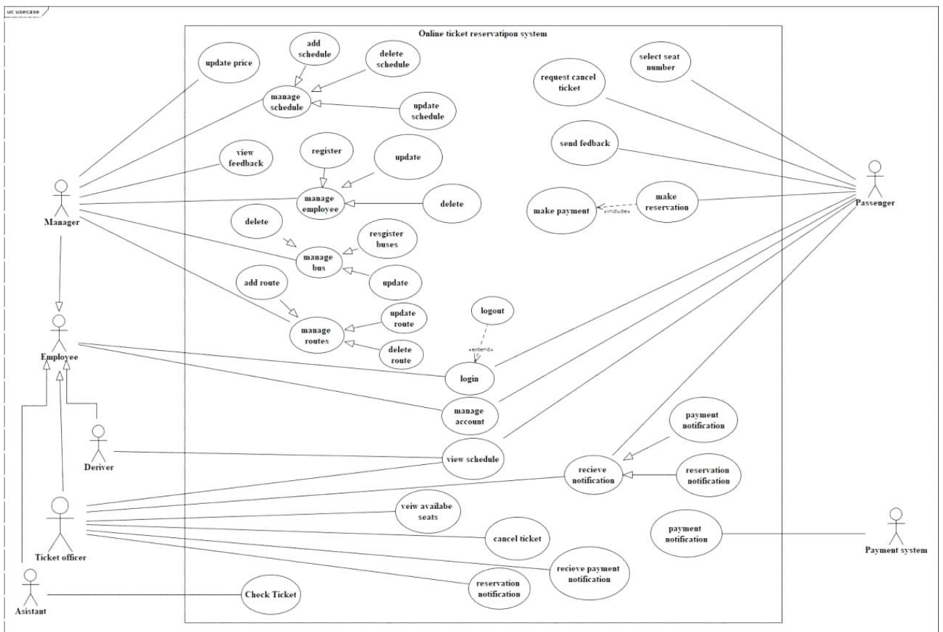
figure 4. 1 use case diagram
