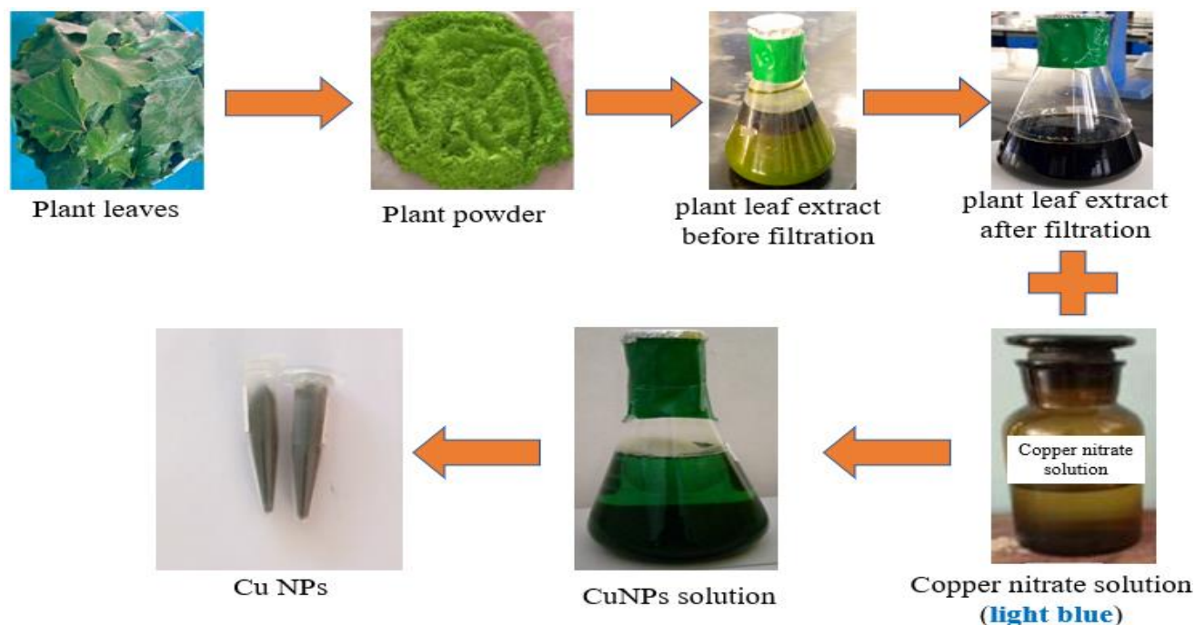
Figure 15: Green synthesis of CuNPs from Xanthium strumarium L. plant leave extract after incubation at room temperature for 24 hrs. And colour change observation.
