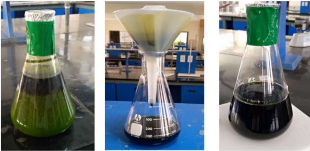
Figure 22: Filtration (Filtering the macerated aqueous PLE to get pure and clear PLE)
