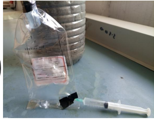
Figure 8 Measurement of gas produced by syringe protocol method
