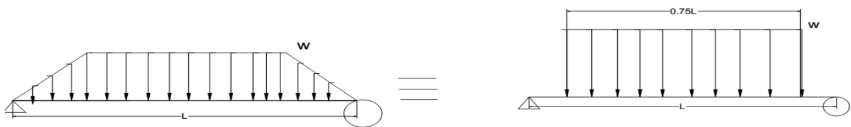
Figure 2-6 Trapezoidal load distribution and its equivalent rectangular load distribution
