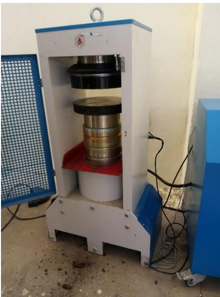
a) Compressive test machine
