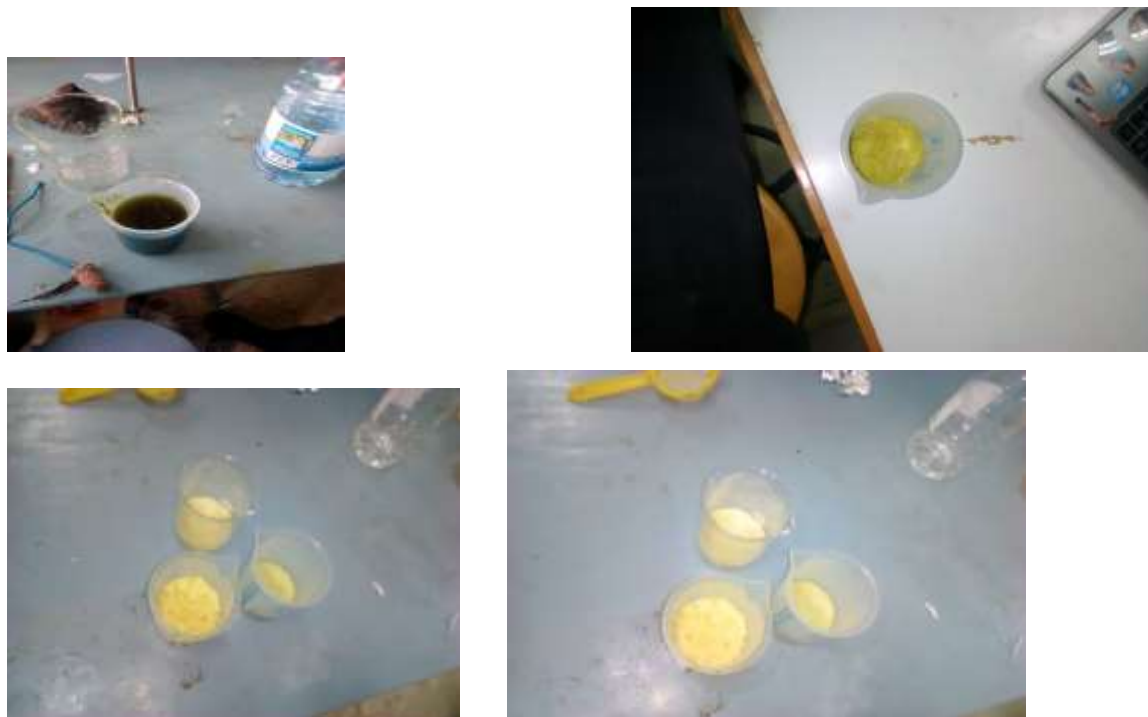
Figure 3 washing, beating and bleaching of pulp
