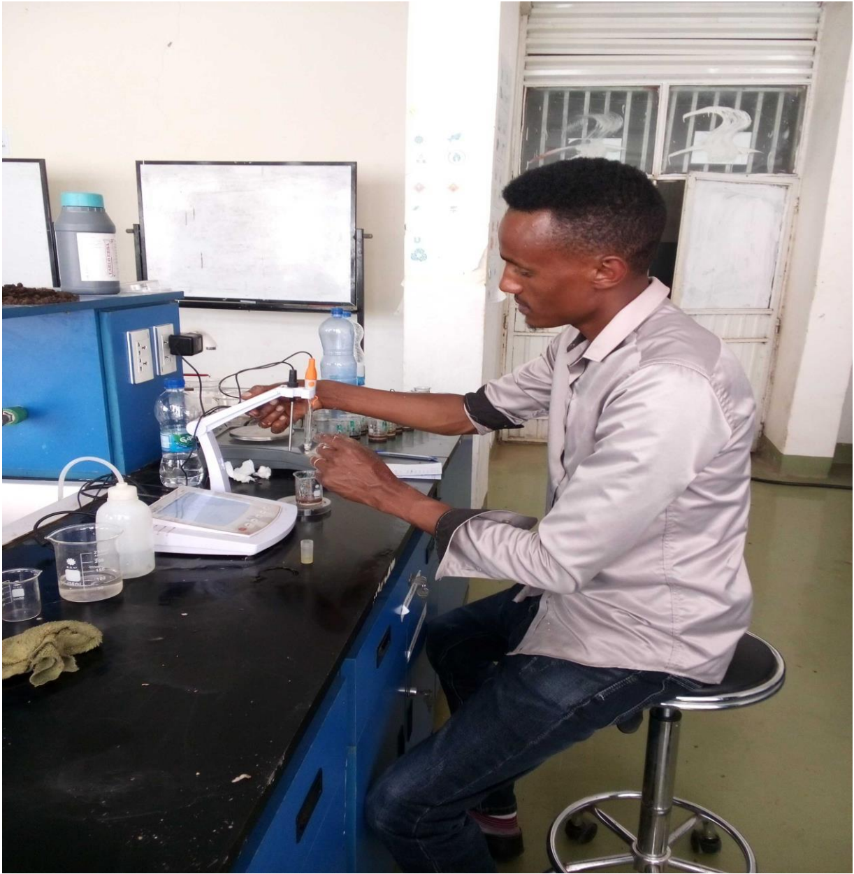
Appendix Figure 5. Testing the pH content of the tuber by using a pH meter
