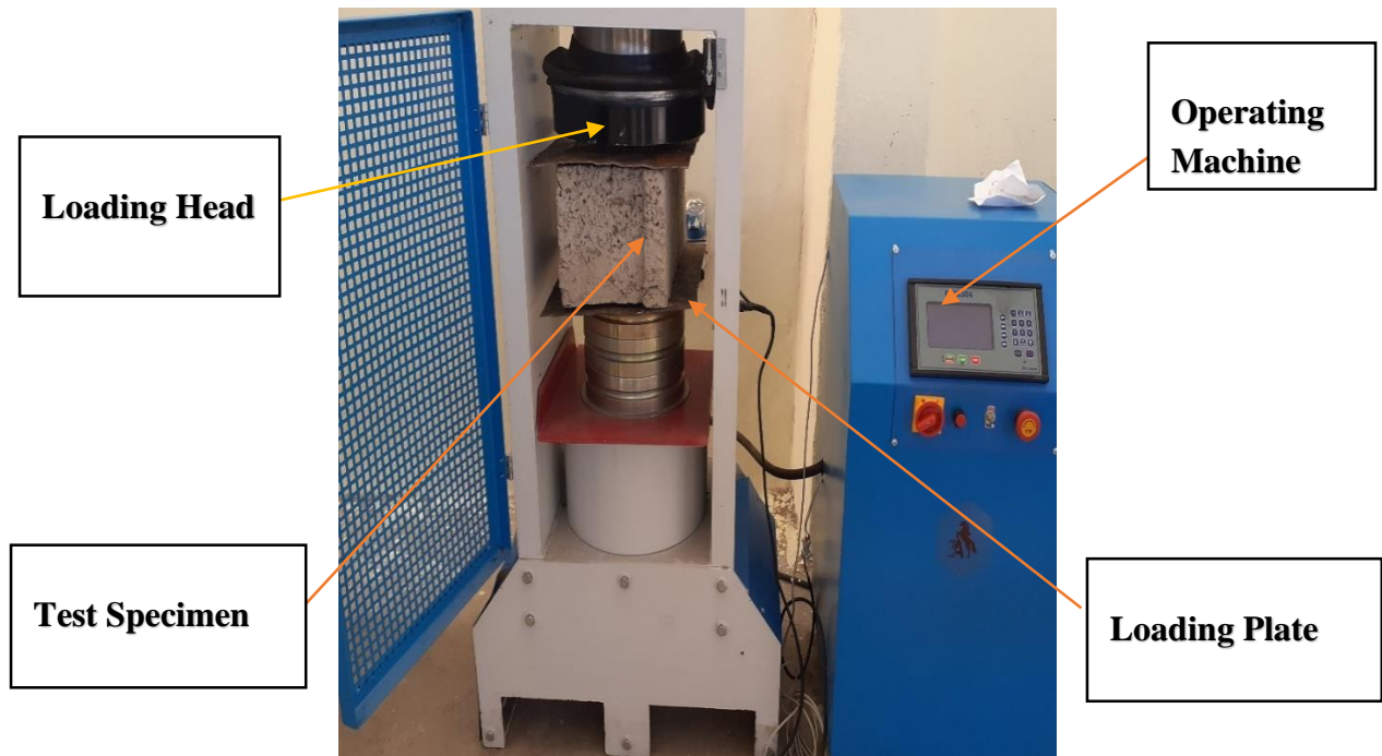
Figure 3-4 Compressive strength test of HCB
