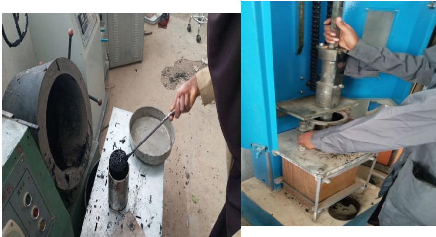
Figure 3.11 aggregate mix and compact
