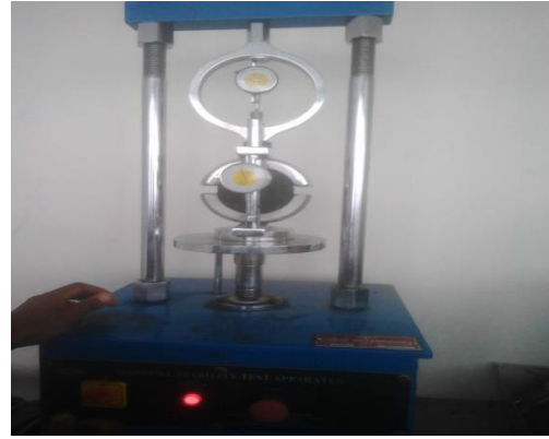
Marshall stability test apparatus
