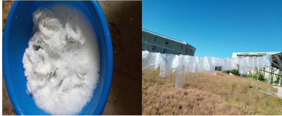
Figure 3.2 Washing and drying of waste plastics
