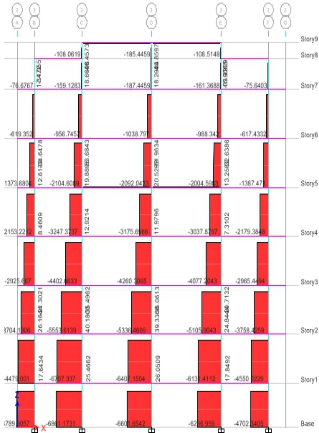
Figure 5. 5 Axis 3-3 And Axis D-D Axial Force Diagram
