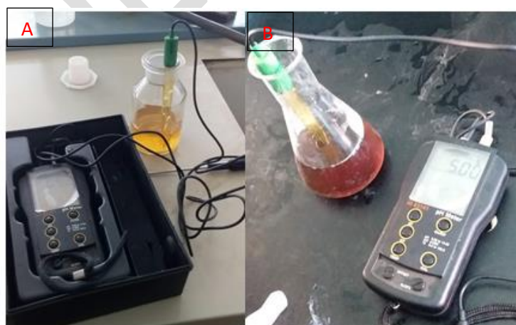
Figure 3.4 PH Adjustment, (A) before PH is adjusted, (B) after PH is adjusted
