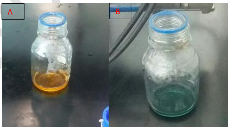
Figure 3.6. Identification of bioethanol, (A) before adding H 2 SO 4 , (B).After adding H 2 SO 4 .
